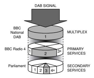
Each multiplex is transmitted in a set frequency range and received by this unit for decoding. You can receive multiplexes broadcast in the 174–240 MHz frequency band and store the services in each multiplex for you to access. The number of multiplexes you receive depend on your location. Channels used in the UK are in the range 10A to 12D.
